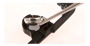
18. Use the tweezers to remove the **Earpiece Gasket** from its compartment.
