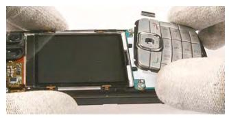
5. Protect the **LCD** with a plastic film.
