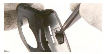
10. Protect the Camera Bezel with a plastic film before turning the unit.
