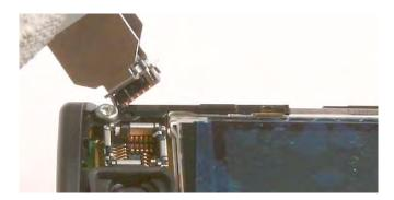
**Note:** When reassembling, note the correct position of the **Camera** when fitting it back into its compartment.
