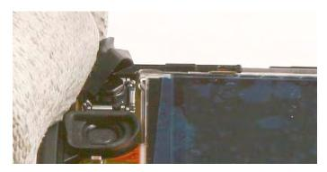
12. Unlock and remove the VGA Camera with the SS-51 camera removal tool.
