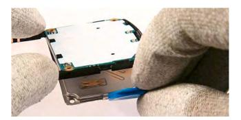
21. To unlock the **UI PWB** from the **UI Frame**, carefully pull the PWB upwards.
