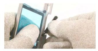
Insert **SRT-6** between the **Antenna Cover** and Chassis, and open the **Antenna Cover** clips. 8. **Note:** Additional force may be required to open the clips.
