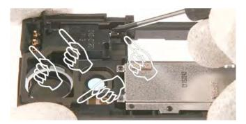
29. Carefully separate the **Antenna** from the **UI Frame**.
