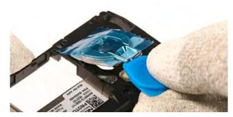
31. Use **SRT-6** to completely remove the residues of the **Camera Rear Bezel Assy** adhesive. Note: When reassembling, always use new adhesive.
