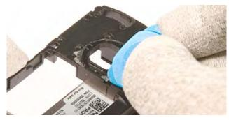
32. To prevent mechanical stress to the PWB, place the **Engine Module** onto **RJ-94**, and use **SS-15** to remove the **Camera** module.
