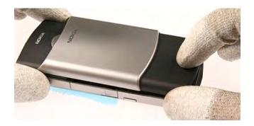
3. Place **SRT-6** between the **A-Cover** and Chassis; release the 4 plastic clips beginning from the bottom side as shown.
