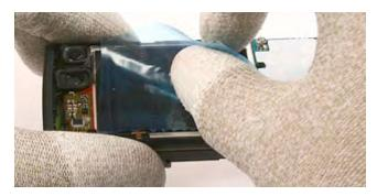
6. Protect the inner side window of the **A-Cover** with a film.
